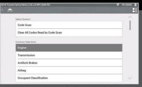
One Touch Code Scan & Clear - Quickly performs checks and completes full vehicle clear codes for all available modules if supported by the vehicle.
