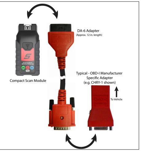
Figure 3-3 OBD-I DA-6 Connection Example
