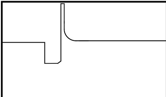
Fig 4. INJector pulse signal
