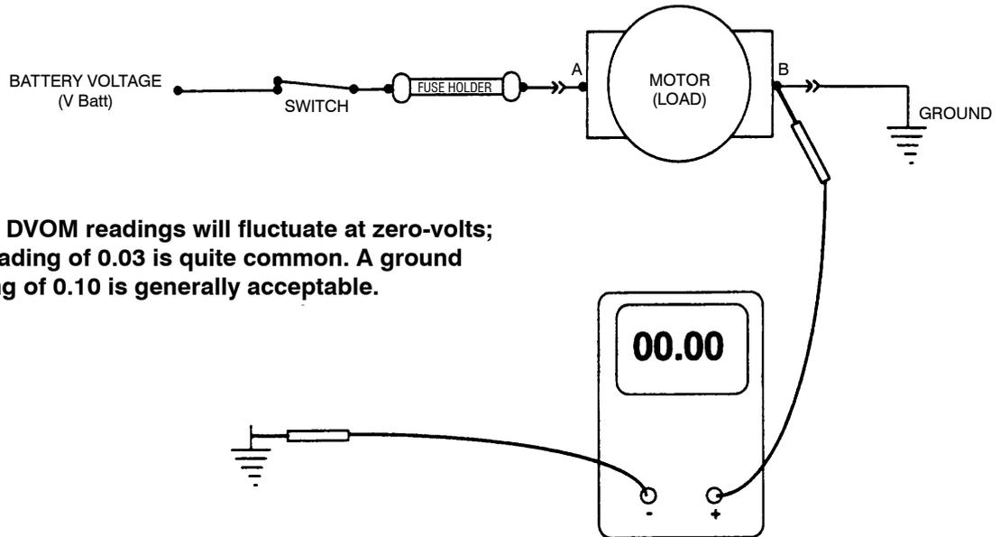
**Note: Most DVOM readings will fluctuate at zero-volts; a DVOM reading of 0.03 is quite common. A ground side reading of 0.10 is generally acceptable.**
