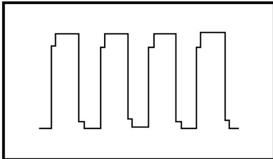
Fig 2. Profile Ignition Pickup signal
